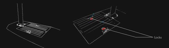
2. Pull the battery out of the board cavity by pulling and gently rocking it side to side.
