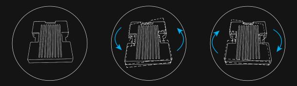
3. Make sure to pull the battery equally from both sides.
