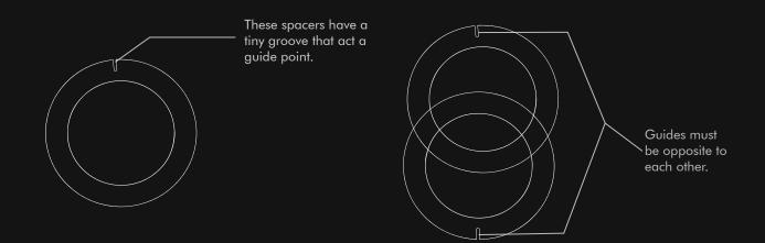
There are guide points on the spacers as shown in the figure above. Place both spacers flat on top of each other with guide points vertical and in the opposite direction of each other.
