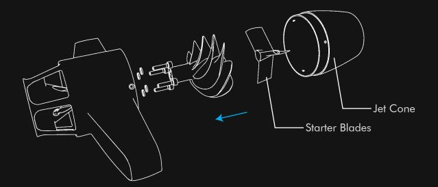
6. Place the cap to the prop guard as depicted in pic and screw it with the screws provided.7. Use 3 x M3 screws to fix the jet cone in place.
