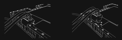
3. Plug in the charger cable to the socket. The typical charge time is 4 hours on standard charger and 2 hours on the fast charger.
