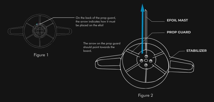
2. Align the prop guard as depicted in figure 2. Ensure the stabilizer is parallel to the floor and the bar of the prop guard aligns vertically with the mast. Once the prop guard is aligned, screw it in place with the screws provided.
