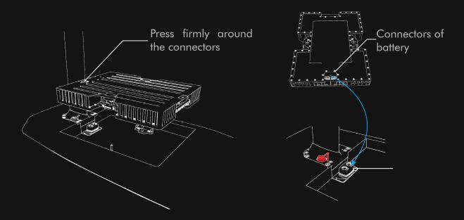
Press the battery near the connector and ensure it's flush with the bottom board surface before screwing it down.
